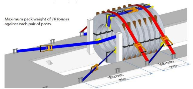
Note: This document displays the minimum restraint requirements for slit coil packs up to 8 tonnes.
