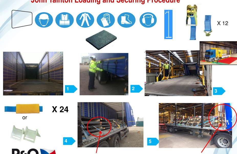
Intermediate straps on each stack
