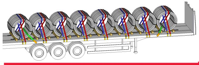
When the Severe Winter Weather Warning is in force anti-slip matting must be placed underneath each cleat.
