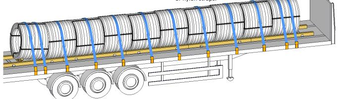
This Load Restraint Guideline is designed and tested to meet the forces specified in EN 12195-1:2010 and VDI 2700 for road and sea transport.
