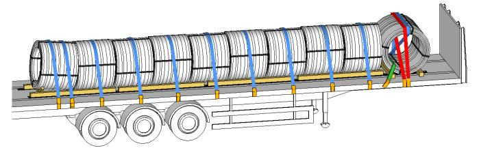
When the Severe Winter Weather Warning is in force anti-slip matting must be placed underneath each timber.
