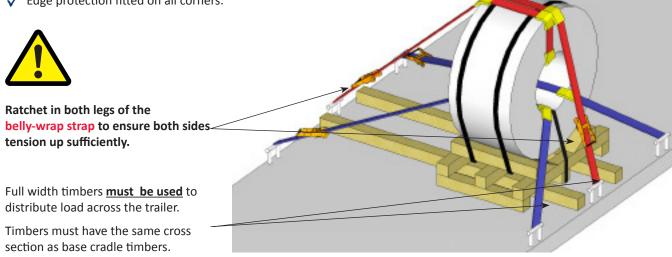
NOTE: Outside diameter (OD) must be less than 3 times sheet width (SW).
