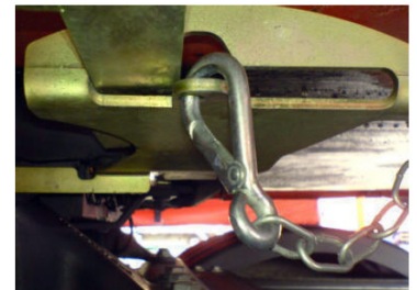
Dog clip fitted through hole in the plate beneath the locking arm.
