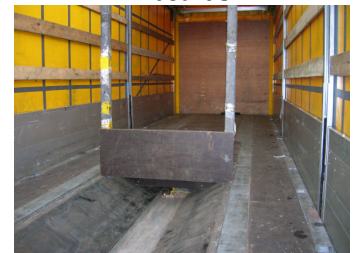
Clean and tidy coil well
