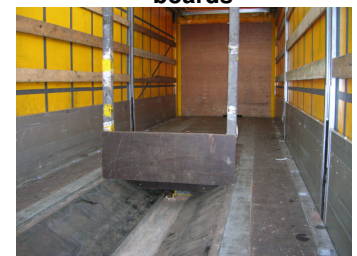
Clean and tidy coil well
