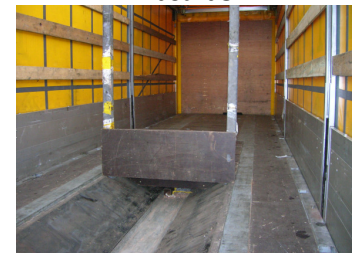
Clean and tidy coil well
