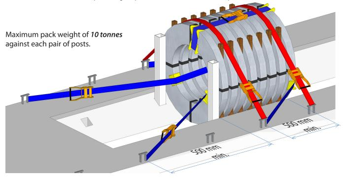
Note: This document displays the **minimum** restraint requirements for slit coil packs up to 8 tonnes.
