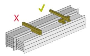
Do not double stack timbers in line, and do not balance timbers on the flanges of beams - create a stable grillage to fill the void.
