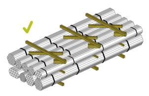
Place packing pieces at an angle to prevent upper timbers sliding off.
