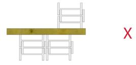
Intermediate dunnage must span the full width of the product below it:
