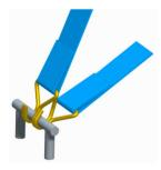
Capacity of webbing strap is reduced by 50% when both ends of the same strap are attached to the same anchor point.
