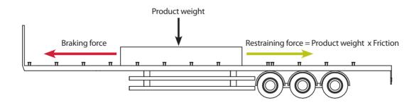
High friction creates more efficient and effective load restraint systems. Some typical friction coefficients are listed below:
