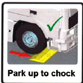
Truck park or loading bay sloping down at front of bay fitted with ground chocks 800 x 800 mm
