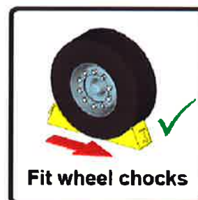
Parking areas with slope exceeding 1:100, with no fixed ground chocks 800 x 800 mm
