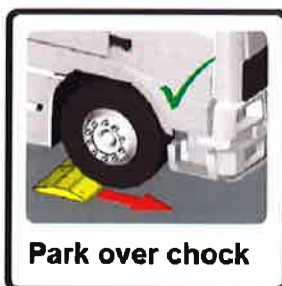
Truck park or loading bay sloping down at rear of bay fitted with ground chocks 800 x 800 mm
